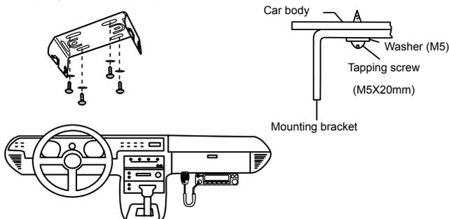
2. Position the transceiver, then insert and tighten the supplied hexagon SEMS screws.
