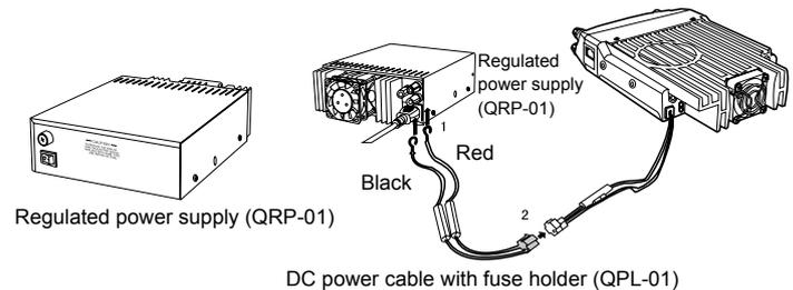
2. Connect the transceiver's DC power connector to the connector on the DC power cable.
